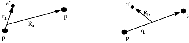
FIG. 1. The Jacobian coordinate systems used. The origin of R_i is at the center of mass of the two particles connected by r_i .
